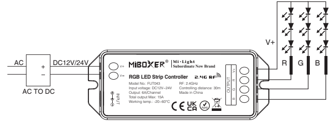
Controller connect to RGB LED strip diagram
